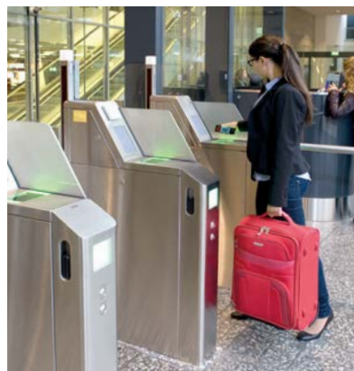
The boarding pass control sensor barrier allows passengers access to airside, before the security checkpoint, with printed or mobile device boarding pass.
