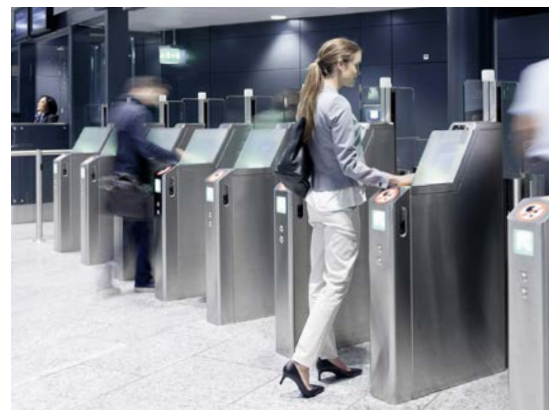
The extended sensor system quickly processes boarding pass information and safely admits one passenger at a time and detects luggage.
