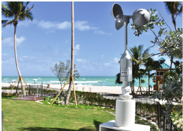
An anemometer monitors wind speeds and provides data to a programmable logic controller (PLC), which in turn sends an input signal to a wind-dampening module mounted directly on each in-ground auto door operator.
