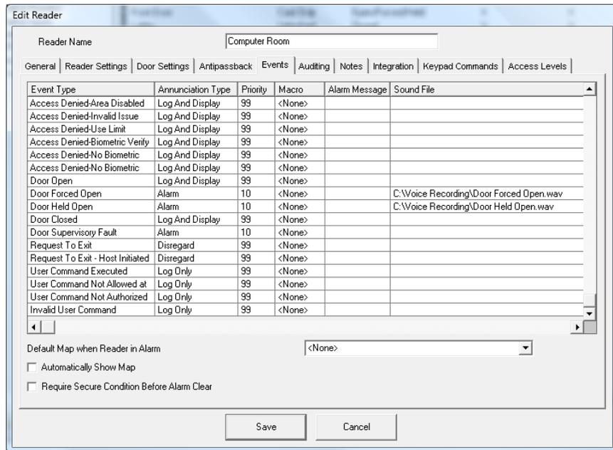
Figure 1: As shown on this screen from RS2's Access It!® Universal software, users can substitute a .wav file of a voice recording in place of a standard Windows® tone.
