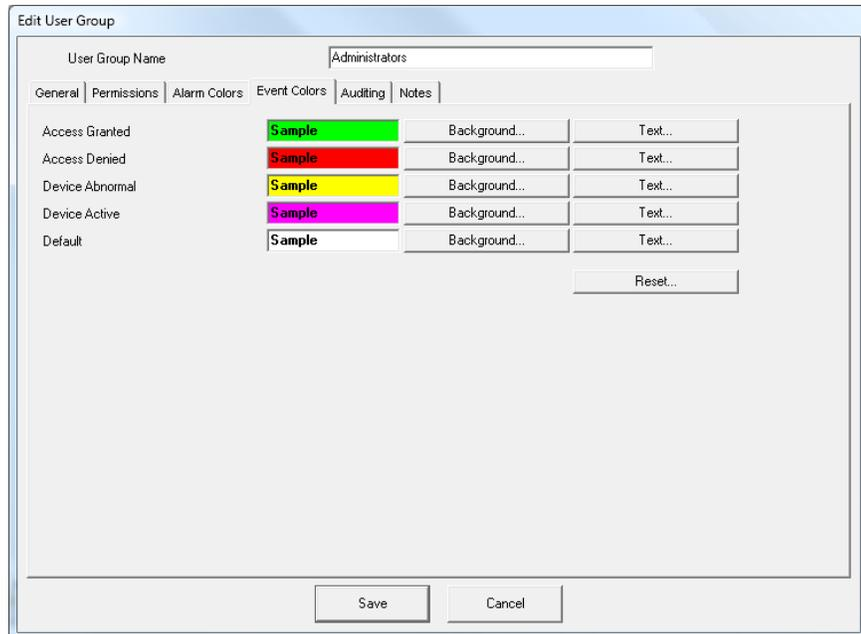
Figure 3: As shown on these screen from RS2's Access It!® Universal software, users can color code alarms or events to indicate priority, importance, or some other criterion.
